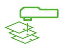
The 2.5D marking head is equipped with an optical focus point adjustment, which enables a quick change of the marking level. A built-in focus point adjustment enables a simpler and cheaper mechanical design for those applications where Laser focus point adjustment is mandatory. The 2.5D marking unit is the recommended solution when the marked object contains several different marking surfaces or mechanical construction is desired to be fixed while product height varies.
